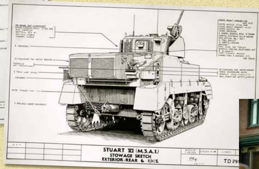
Sketches of the M5A1 Stuart as produced for the British Army, with right the characteristic extra stowage mounted on the back of the tank.
