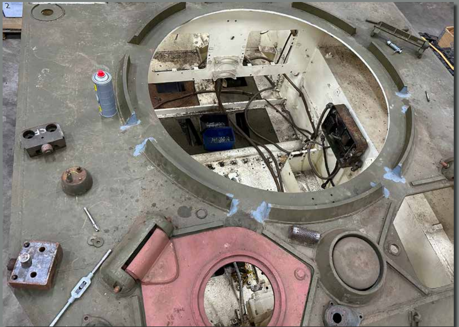
Trial fitting turret rollers and first CAD-design for reproduction
