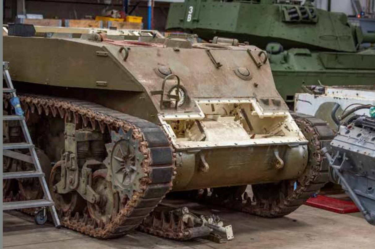
Start of dismantling the M5A1
