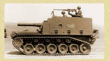
First of all they adopted an open-air hull structure to dispose of the toxic gasses when firing. The open hull also gave a better working space for the crew and provided natural light, though the crew was more exposed to battlefield dangers.
