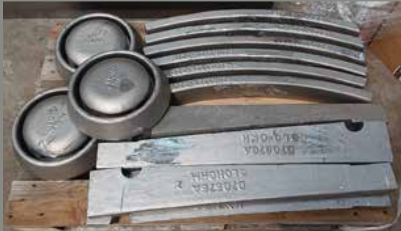
Casting moulds for reproduction of bullet catchers around the base of the turret
